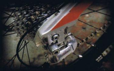
Splined adjustable dropouts
