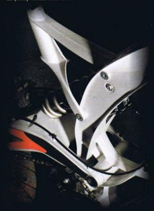
Bolt-on seat mast above regular sized pivot bearings
