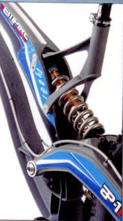
One-of-kind: The AP-1R frame uses a single-pivot suspension and Cane Creek Double Barrel shock.
