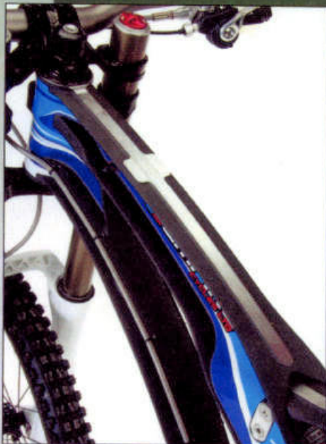
The top tube's ground-down "seam" from where the sand-casting molds come together.
